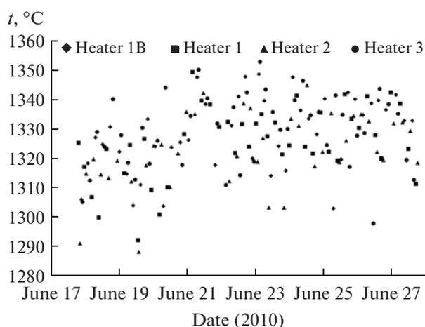
Fig. 3. Cupola temperature at the end of the gas period.
