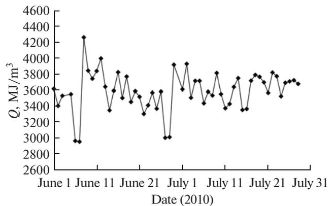
Fig. 2. Fluctuations in calorific value of blast-furnace gas.
