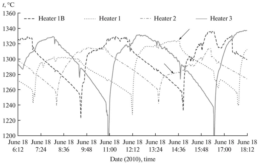
Fig. 4. Cupola temperature in blast heater on June 18, 2010.
