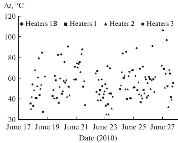
Fig. 8. Difference in the temperatures at the beginning and end of the blast period.
