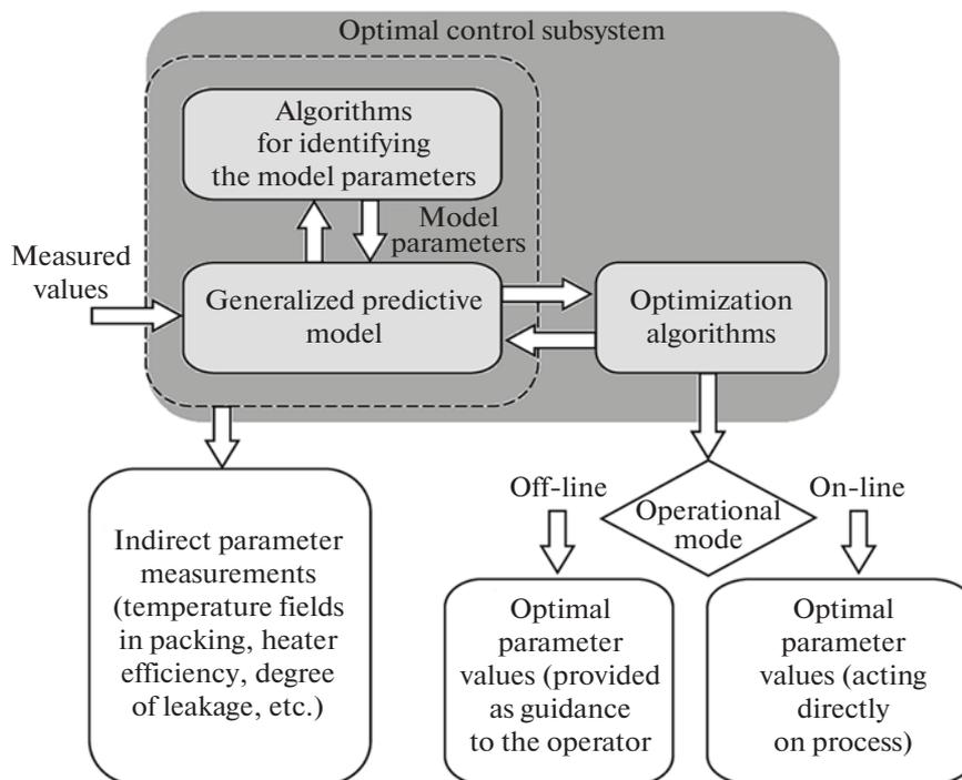
Fig. 1. Structure of the optimal control subsystem.
