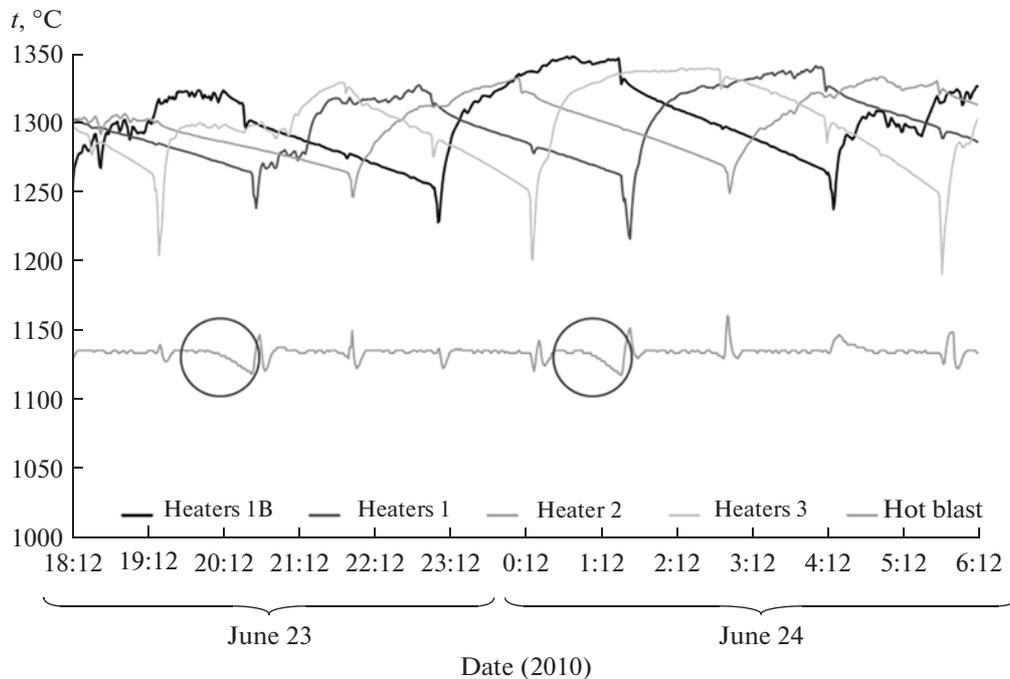
Fig. 9. Cupola temperature and hot-blast temperature.
