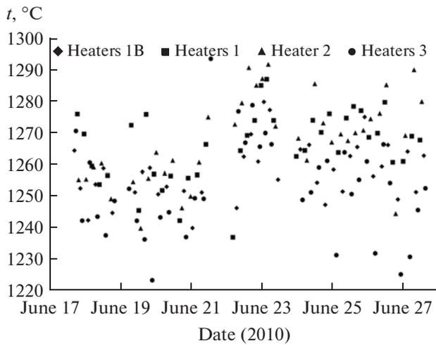
Fig. 7. Minimum cupola temperature at the end of the blast period.
