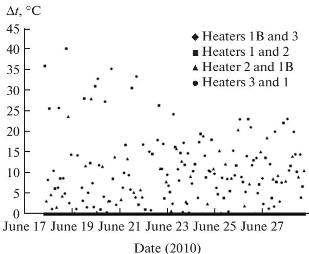
Fig. 5. Difference in the cupola temperatures for different pairs of blast heaters operating with gas (at the end of the gas period of one heater).
