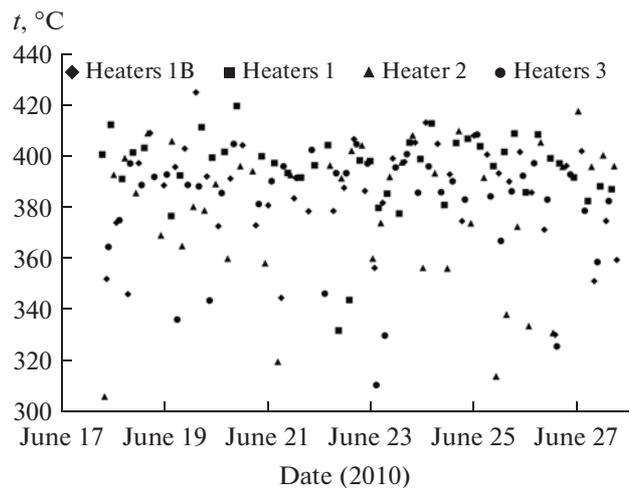
Fig. 6. Exhaust-gas temperature within the heater at the end of the gas period.
