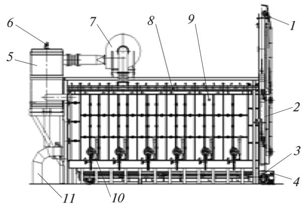
**Fig. 1.** Side view of furnace: 1) mechanism for raising door; 2) mobile guides for door-clamping mechanism; 3) drive of hearth-sealing mechanism; 4) rolling hearth; 5) portable heating chamber for exhaust gas; 6) burner for portable heating chamber; 7) recirculation fan; 8) roof panels; 9) side panels; 10) exhaust channel; 11) primary burners.
