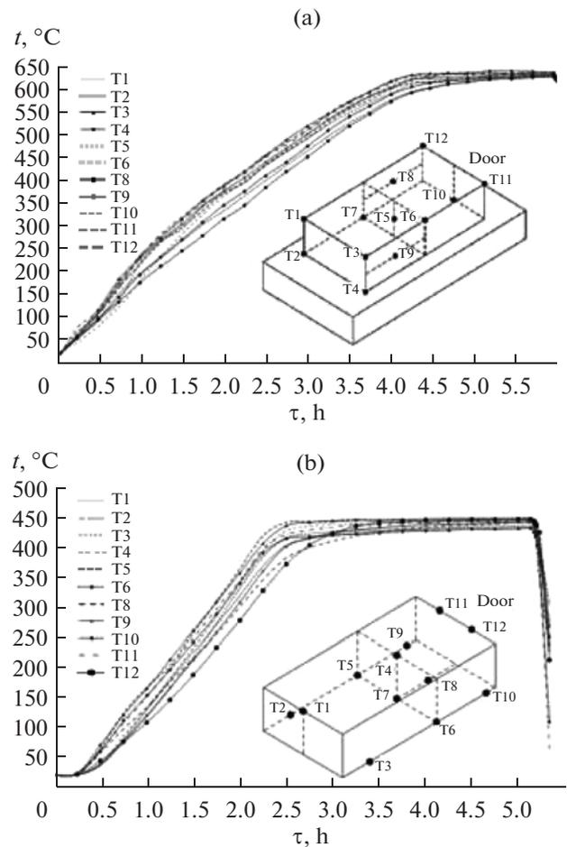
Fig. 5. Heat treatment of components 1 (a) and 2 (b).
