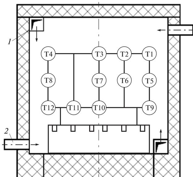
Fig. 2. Configuration of thermal converters on the moving frame: 1) line supplying recirculated gas; 2) burner.
