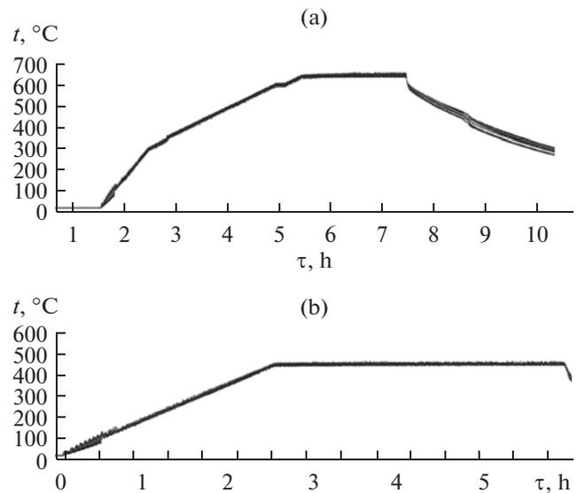
Fig. 4. Heat treatment of components 1 (a) and 2 (b).
