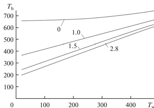
**Fig. 3.** Calculated dependence of the coil temperature on the mean temperature of the housing walls for a 55-kW heater; the values of the fan productivity ( $m^3/s$ ) are given on the curves.
