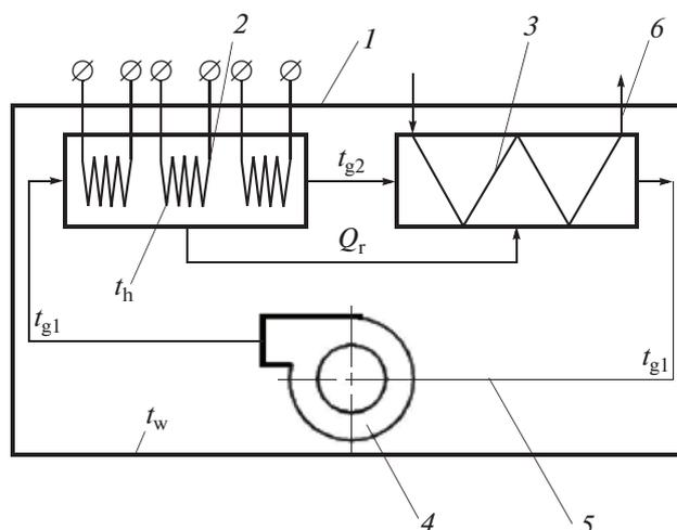
**Fig. 1.** Heat transfer in a closed electric heater with radiant–convective heat transfer from the coil to the housing: 1) sealed protective housing; 2) heating coil; 3) tubular heat exchanger; 4) high-temperature fan; 5) input and output channels; 6) hot dirty air. For further explanation, see the text.
