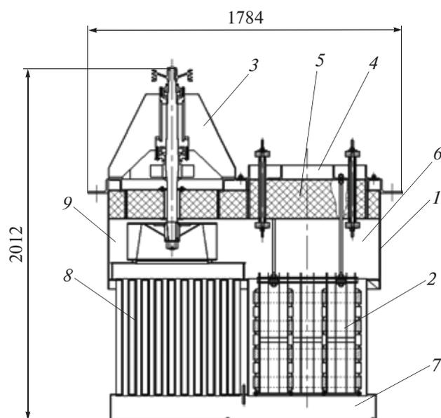
**Fig. 2.** Closed electric heater with radiant–convective heat transfer: 1) housing; 2) suspended attachment system for heating coils; 3) custom-designed circulatory fan; 4) supporting flange; 5) heat-insulating layer; 6, 7) upper and lower passageways; 8) tubular heat exchanger; 9) built-in helical fan housing.
