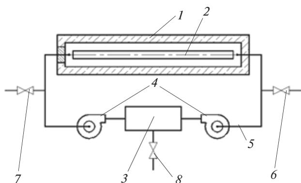
**Fig. 1.** Convective furnace with a complete heat-transfer cycle and periodic reversal of the gas motion, for the heat treatment of long parts: 1) furnace housing; 2) long part; 3) heater; 4) reversible device; 5) connecting channels; 6, 7) coolant (air) supply; 8) coolant extraction.
