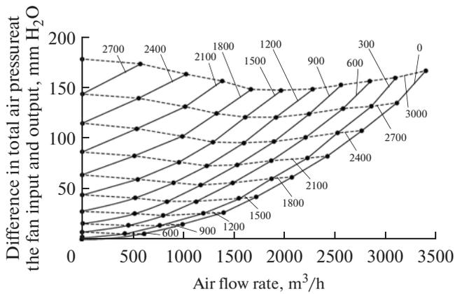
**Fig. 3.** Experimental aerodynamic characteristics of the reversible device in conditions of aerodynamic closure (air density  $\rho = 1.2 \text{ g/dm}^3$ ) for the counterflow fan (continuous curves) and blast fan (dashed curves), in the case of Ts14-46 2.5 fans; the fan speeds ( $n$ , rpm) are given on the curves.
