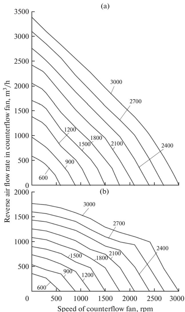
**Fig. 4.** Experimental control characteristics of the reversible devices based on the Ts14-46 2.5 fan (a) and Ts3-81 2.5 fan (b) in conditions of aerodynamic closure; the fan speeds ( $n$ , rpm) are given on the curves.
