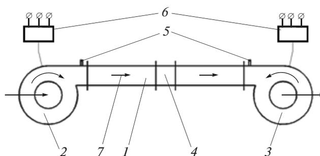
**Fig. 2.** Test bench for the investigation of centrifugal fans operating with aerodynamic regulation of the air flow: 1) pipeline; 2) blast fan; 3) counterflow fan; 4) flow meter; 5) pressure sensors; 6) frequency converters; 7) direction of air motion.
