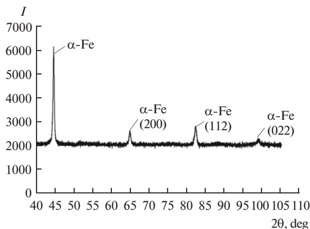
**Fig. 6.** X-ray diffraction pattern from the middle section of the fishtail's neck:  $I$ , intensity;  $2\theta$ , disorientation angle.
