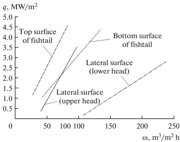
Fig. 4. Dependence of the heat-flux density on the irrigation density according to experimental data for the top, bottom, and lateral surfaces of the fishtail in an industrial system.
