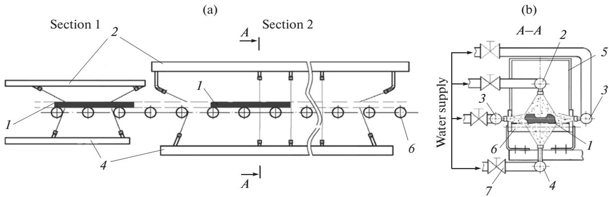
**Fig. 1.** Side view of controllable cooling system for fishtails (a) and a single cooling loop (b): 1) fishtail; 2) upper supply line; 3) lateral supply line; 4) lower supply line; 5) protective housing; 6) rollers; 7) valve.
