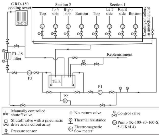
Fig. 3. Water-supply system to the quenching unit at OOO NSMZ.
