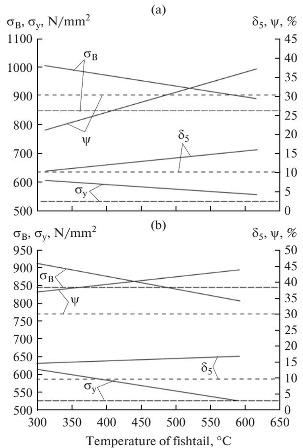
Fig. 5. Experimental (continuous curves) and standard (dashed curves) dependence of the strength and plasticity of fishtails with 0.56–0.57% C (a) and 0.485% C (b) on the final temperature in spray cooling.
