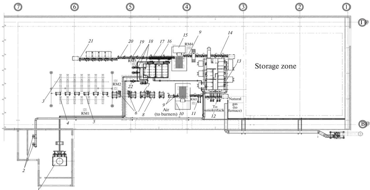
**Fig. 2.** Department for quenching of fishtails at OOO NSMZ: 2) furnace fan; 6) tipping system; 7) roller conveyor for inspection of blank; 11) reversing unit; 12) furnace-charging conveyor; 14) discharge roller conveyor; 16) water tank; 18) pumps; 19) tipping unit; 20) roller conveyor. The other notation is explained in the text.
